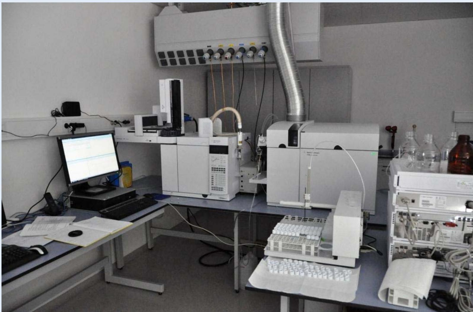
ICP-MS Agilent 7700x with GC and HPLC separation system
